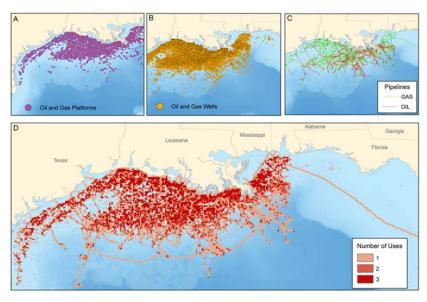
Figure 2: Location of present-day key oil and gas infrastructure in the Gulf of Mexico; Oil and Gas Platforms (A), Oil and Gas Wells (B), and Pipelines (C). Cumulative number of oil and gas ocean use activities per 4.77 x 4.77 km grid cell in the Gulf of Mexico (D).
